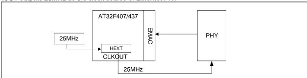
2. 25MHz is directly used as the clock source of Ethernet PHY.
