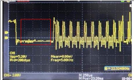
The USART receive side being low prior to USART enable would cause MCU to receive 0x00 (receive error) as long as USART is enabled.
