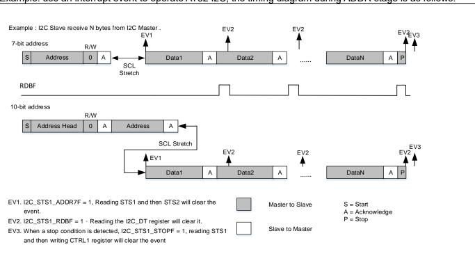
It can be seen from the figure above that slave enters interrupt after detecting a correct ADDR on EV1 event, and releases SCL line only after ADDRF flag bit is cleared by reading status registers STS1 and STS2. If this is the case, this operation may cause unwanted problems. As a result, one of the more reliable ways is to let slave releases SCL line before the SCL is controlled by master. This can be done by modifying master code or slave code.
