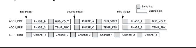
When ADC1 ordinary group is converting, an attempt of switching from ordinary group to ADC1 preempted group would cause conversion error in ordinary group.
